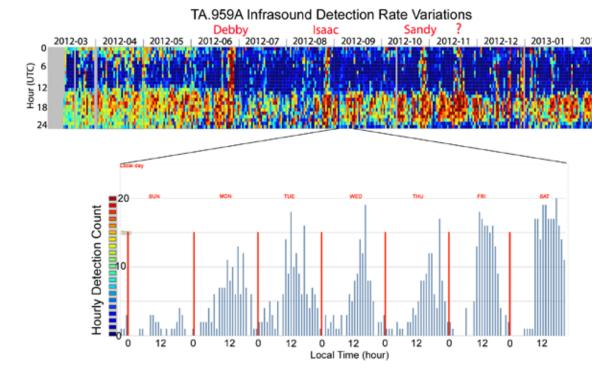
Figure 2. Plots of TAID detection rate (number of detections per hour) for TA station 959A near Okeechobee, Florida. Variations in detection rate are an indicator of the noise level at the station. Upper plot is a one-year 3-D detection rate plot with color representing detection rate.
