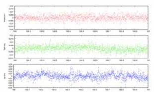
**Figure 2.** Kinematic processed baseline positions between P804 (deep drilled monument) and P805 (short drilled monument) for one 24-hour period (2013 Day 100) using the TRACK software. The baseline residuals for three components North, East, and Up are displayed in meters.
