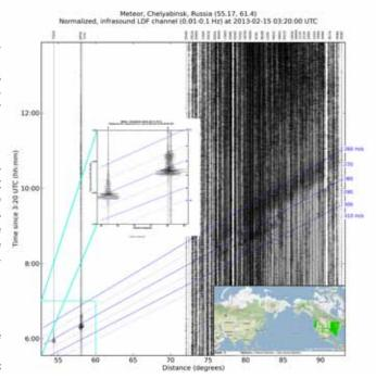
**Figure 1.** Infrasound record section of the TA low-frequency LDF channels for the Russian Chelyabinsk meteorite of 2013-02-15 with a 0.01-0.1 band-pass filter applied. Traces are normalized individually and are arranged based on their distance (in degrees along the horizontal axis) from Chelyabinsk.
