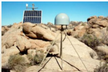
Continuous GPS station PJZX in Baja California with meteorological instrument (on top of solar panel).
