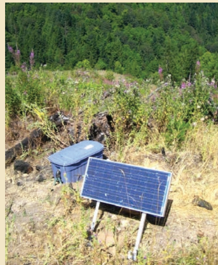
Campaign seismometer deployed to record the episodic earthquakes in the Pacific Northwest.
