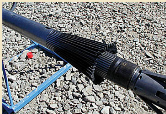
A second 40-arm caliper log confirmed deformation of the borehole casing by the San Andreas Fault.
