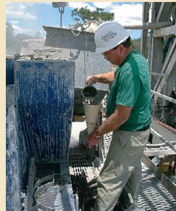
At the SAFOD drill site, A. Bartley performs a routine measurement of the drilling mud properties.
