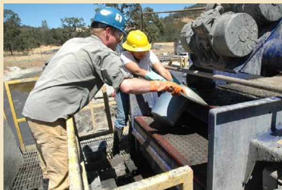
J. Solum and S. Tembe collect cuttings during coring at a depth of 13,091 ft.
