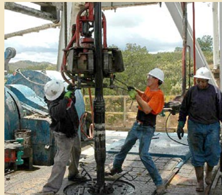
On the rig floor at the SAFOD drill site, the Nabors drill crew pull drill pipe out of the well as drilling resumed in June.
