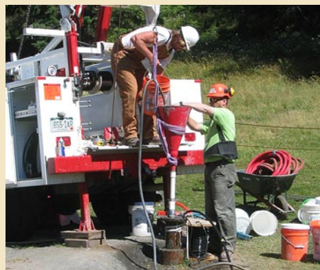
Installing the first EarthScope borehole strainmeter near Hoko, Washington. By the end of June, three borehole strainmeters were completed.
