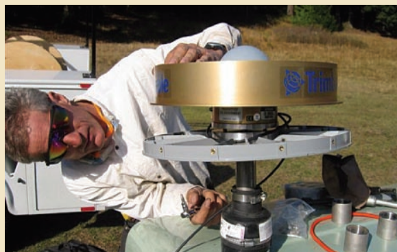
P. Gray attaching the GPS antenna to the borehole strainmeter wellhead.
