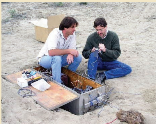
Magnetotelluric instruments will measure electro-magnetic properties at depth.
