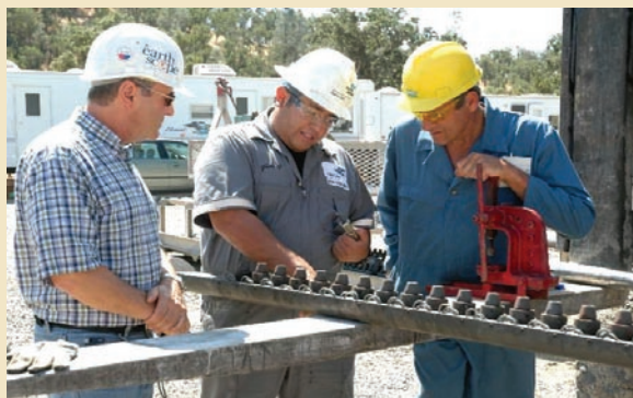
Discussing set-up of the sidewall coring tool. Successful firing of the tool resulted in the collection of 52 cores.
