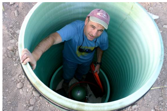
Installation of STS2 inside 36" prototype vault in Socorro, NM.
