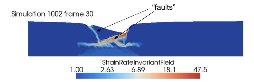
Lower crust is initially 10 km thick Total crust is initially 35 km thick
