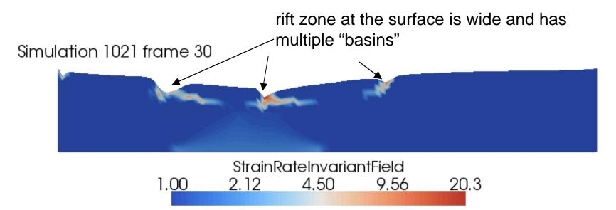
Preliminary result: Start with a thick but not very weak lower crust... (weakening the crust localizes rifting, all other factors being equal) Initial thickness of the lower crust here is 20 km...
