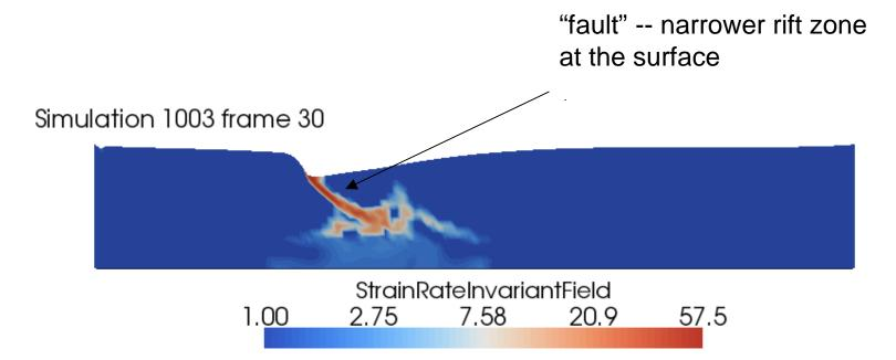
Lower crust is initially 10 km thick Total crust is initially 35 km thick Reduce the strength of the lower crust by a factor 100 (make it very jelly-like!)...
