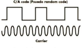
The trick is to find one particular carrier cycle and use it for timing.
