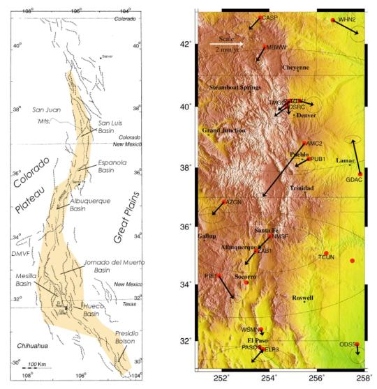
Extension rate not well known – estimates are anywhere from 0.1 mm/yr to 5 mm/yr depending on measurement method
