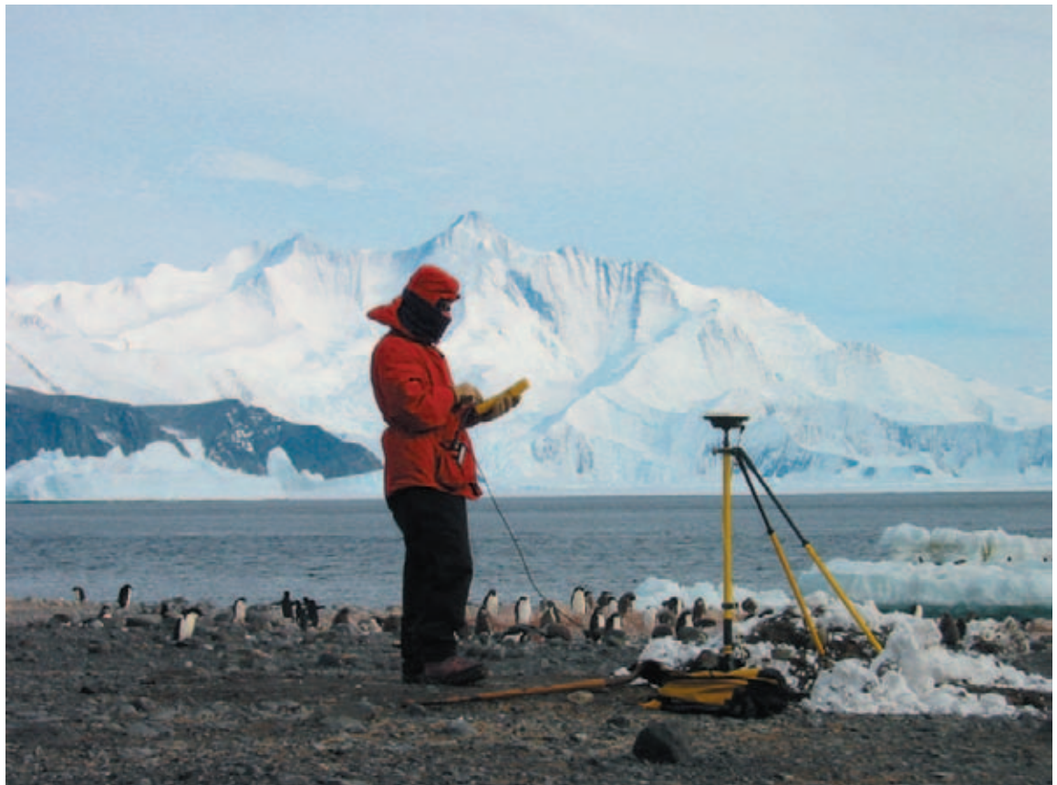
Kinematic GPS survey conducted by Chuck Kurnik (UNAVCO) in support of environmental remediation efforts at Cape Hallett Antarctica. Photo by Geoff Gilbert, Raytheon Polar Services Company.
