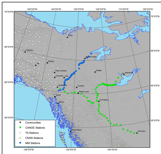
Figure 1. Regional map of present and past broadband seismic stations. The networks included in this map are Transportable Array (white triangles), Canadian National Seismographic Network (yellow triangles), Mackenzie Mountains transect (blue squares) and CANOE (green squares). Note that a subset of these were chosen for our study.
