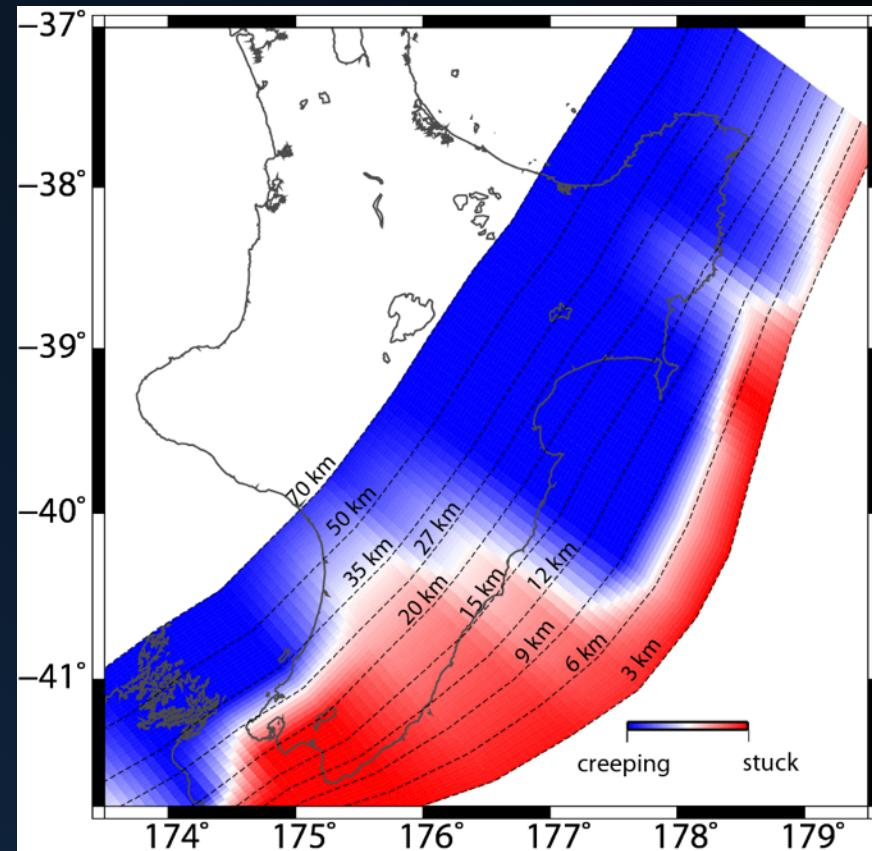
GPS data also reflect long-term tectonic rotation of the forearc. Invert for locking and rotation using elastic block modelling (Defnode; McCaffrey, 2002)
