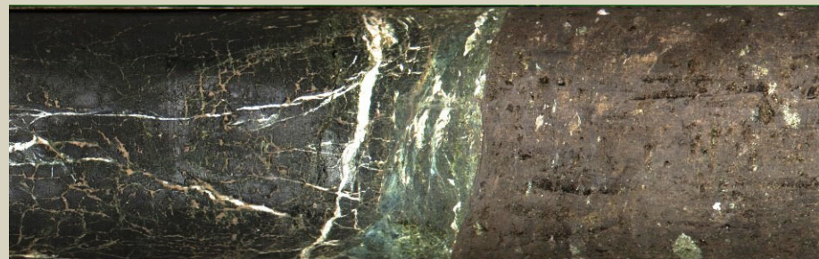
Figure 3: This is a cropped image of core G27 from the Southwest Deforming Zone. Note the transition from black shale, through sheared serpentinite, into foliated fault gouge (left to right). (Zoback et al., 2011).
