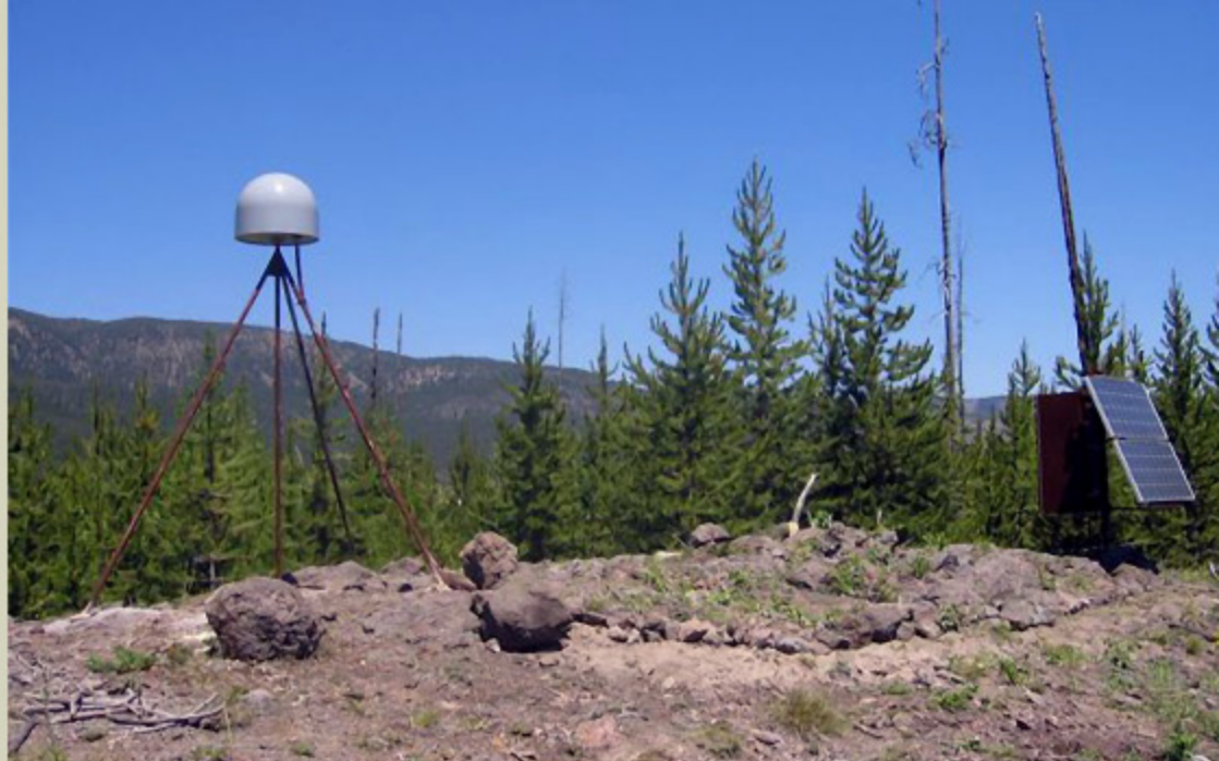
GPS Station P711 - Madison Junction, WY: Located at 110.9W 44.6W, this instrument records ground movement associated with the Yellowstone Hotspot.
