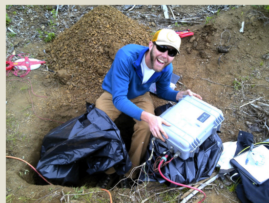
MOCHA MT station MJO11, Yamhill County, Oregon. MOCHA field crew member completing configuration of NIMS Long-Period MT data acquisition system.
