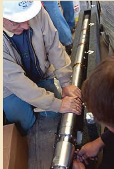
Operations and performance testing on borehole strainmeter in preparation for installation.
