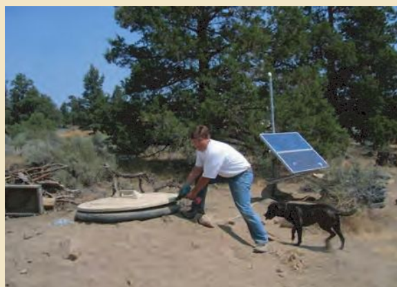
Placing the weather-tight lid on the vault that holds the Transportable Array seismic instrumentation at Bend, OR. Installation of these sites often attracts the interest of local land owners and their animals.
