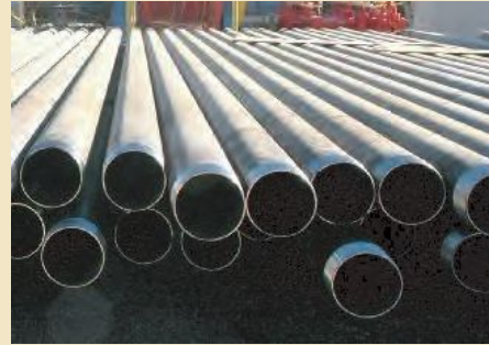
24.4 cm casing for the borehole.
