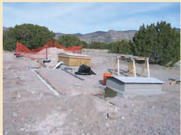
Transportable Array (rear) and ANSS Backbone (front) vaults in parallel test at Albuquerque Seismological Lab.
