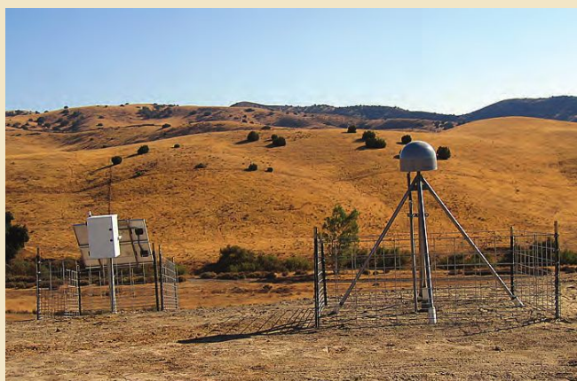
GPS station P532, a deep drilled-braced monument, located southeast of the Parkfield earthquake hypocenter.
