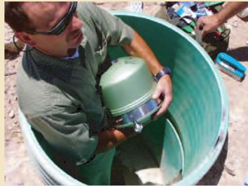
M. Alvarez installing the STS-2 sensor in the Transportable Array site at Socorro, NM.
