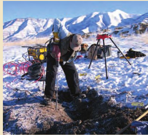
Fred Jenkins drilling holes to install a short drill braced GPS monument located in Lakepoint, UT.
