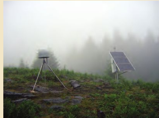
PBO station P170 in Northern California using a short-drilled braced monument style installation
