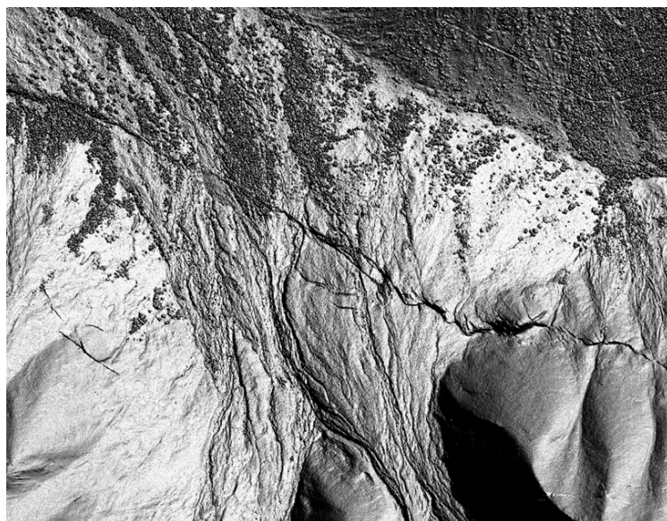
The 2002 Denali earthquake surface rupture crosses alluvial fans, as imaged in EarthScope lidar data.
