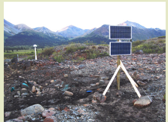
Installed seismometer and continuous GPS site at Macmillan Pass. Photo by Derek Schutt.
